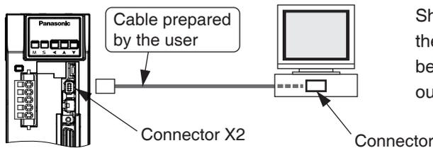
Shut off both powers of the PC and the driver before inserting/pulling out the connector.
