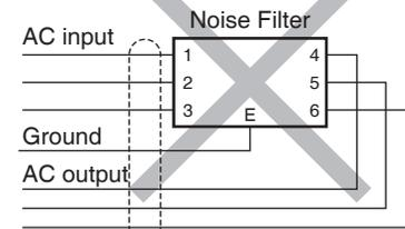
Do not place the input and output lines in the same duct or do not tie both in a bundle.
